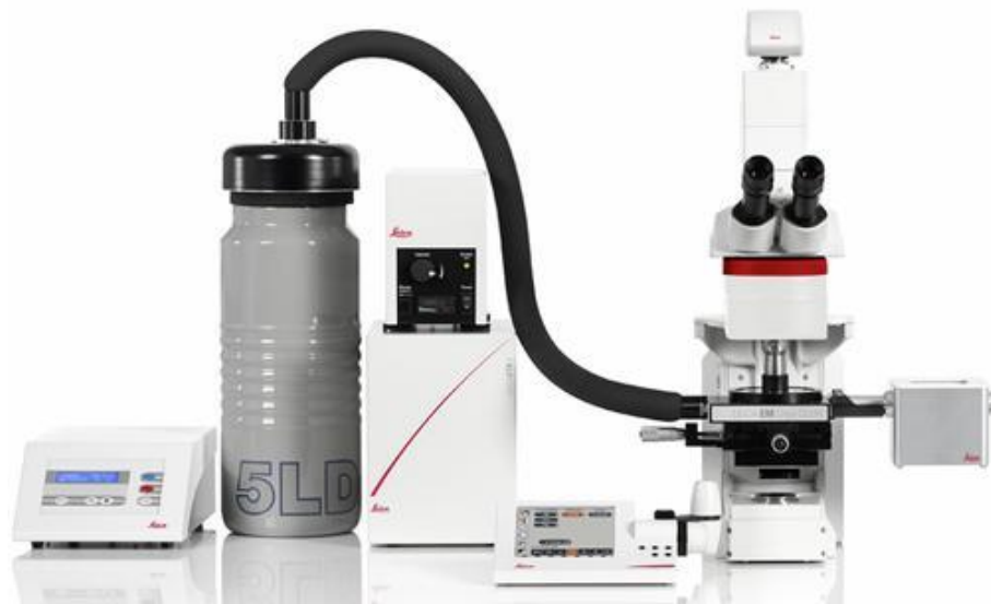
Figure 5-4: Leica Cryo-Stage. Components from left to right: Cooling unit control system, liquid nitrogen tank which pumps nitrogen vapour into the cryo-stage, lamp and power units, microscope control unit and widefield microscope with cryo-stage attachment and transfer system[14].
