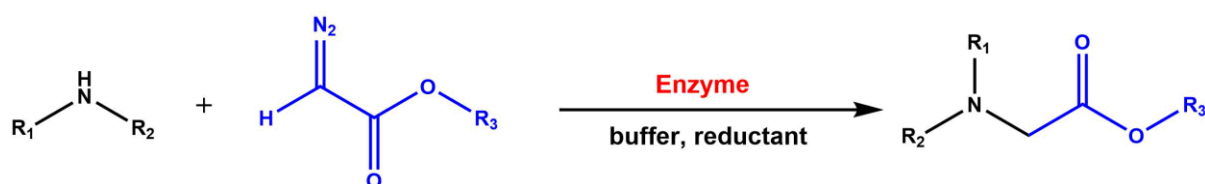
Figure 96: The general reaction scheme for an enzyme-catalysed N-H insertion reaction between a primary/secondary amine and a diazo compound.
