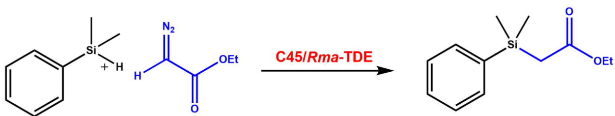
Figure 111: The general C45/ Rma -TDE-catalysed Si-H insertion assay between EDA and DMPS.
