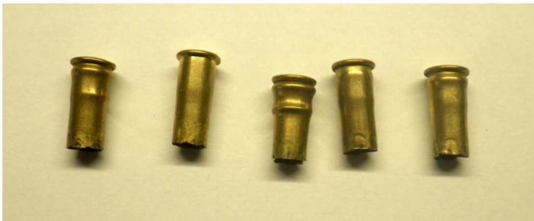
Figure 18. Range of deformities seen in cartridge cases fired using the same device.
