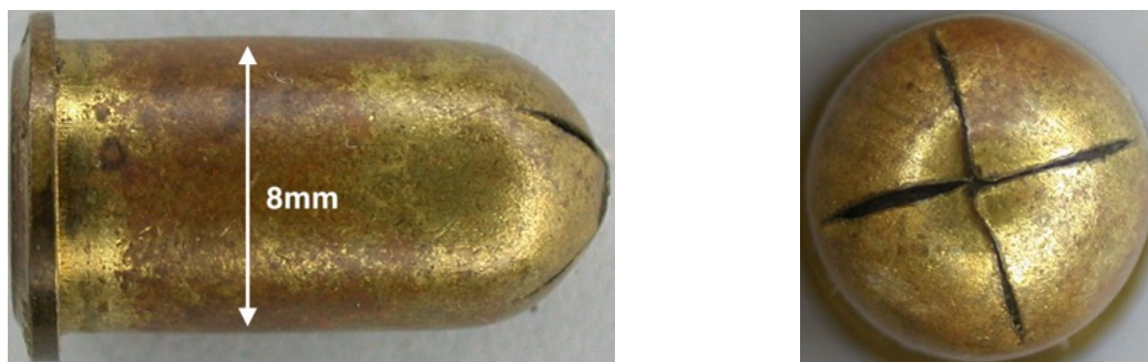
Figure 23: 8mm blank cartridge for Behr cattle killer (municion.org)
