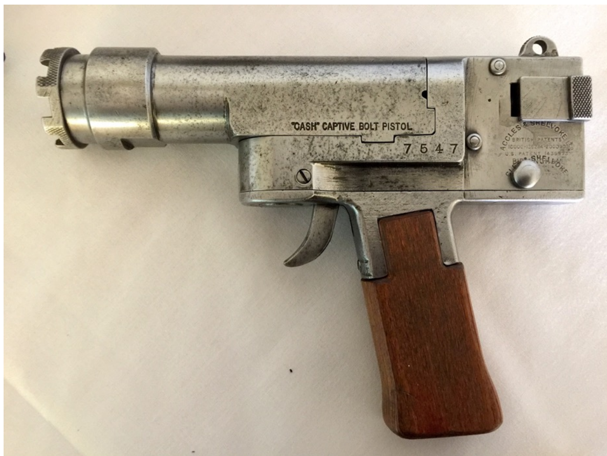
Figure 28: CASH model B Captive Bolt Pistol (Author's collection)
