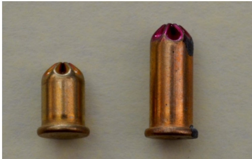
Figure 3. Temple Cox (manufacturer) 0.22" blank cartridges: 1.00 grain cartridge on left; 2.00 grain cartridge on right.
