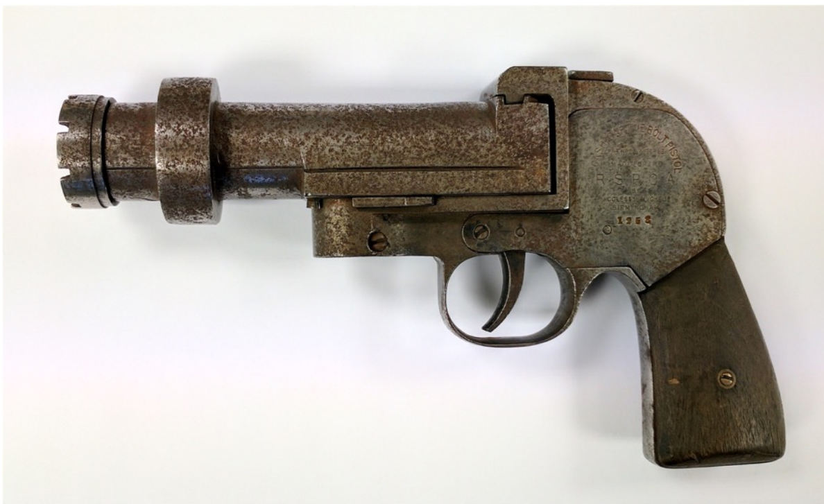
Figure 26: Accles and Shelvoke CASH RSPCA Captive Bolt Pistol (A&S Museum)
