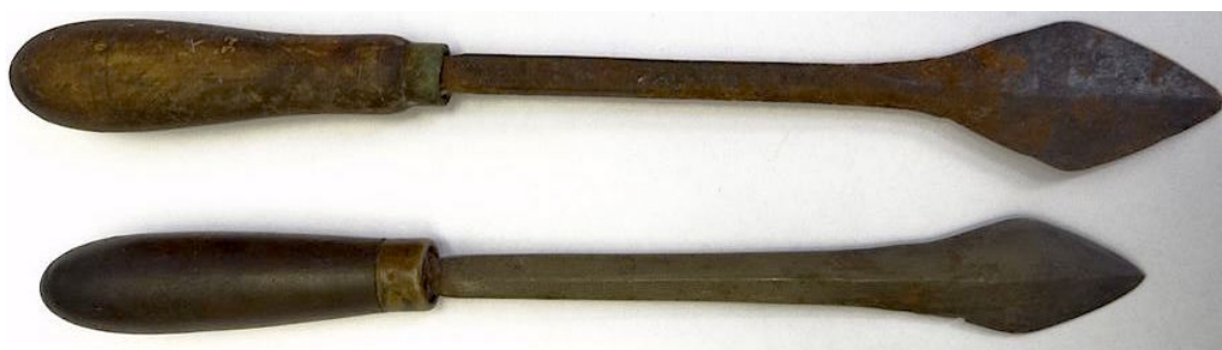
Figure 1: Two nape stab knives with characteristic diamond shape tips
