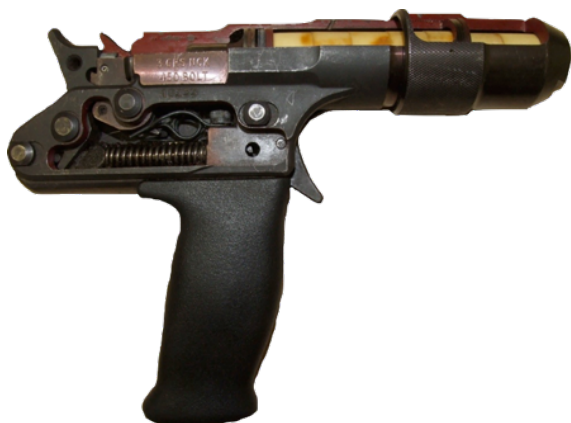
Figure 34. Example of a cartridge powered, trigger-fired penetrating captive bolt device (Split model)
