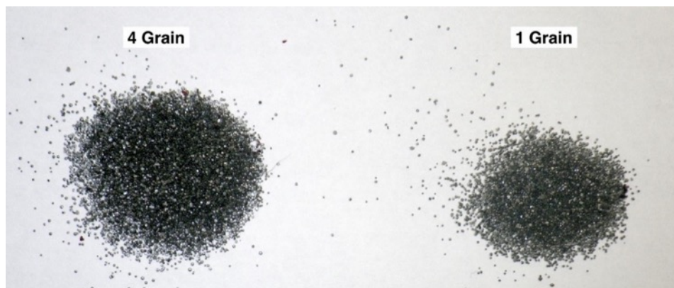
Figure 16. Cartridge contents comparison between a 4.00 grain and a 1.00 grain 0.22” calibre cartridge. Both cartridge cases are the same length and volume.
