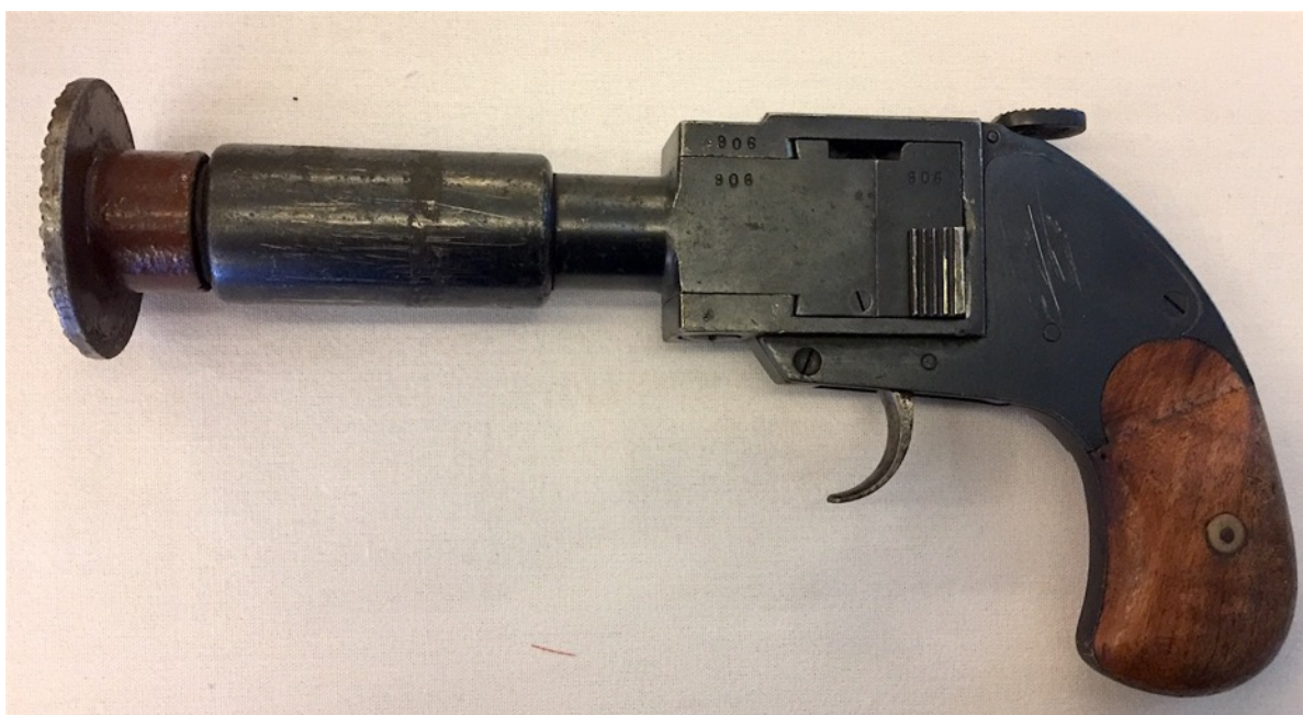
Figure 22: Later model of Behr's "Flash" Cattle Killer with head plate (Author's Collection)
