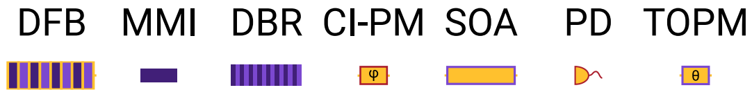
Figure 5.1: List of components used for the chip schematics: distributed feedback (DFB) laser, multi-mode interferometer (MMI), distributed Bragg reflector (DBR), current-injection phase modulator (CI-PM), semiconductor optical amplifier (SOA), photodiode (PD), thermo-optic phase modulator (TOPM).
