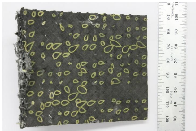
Figure 4-2: An example of loop variation visible on the surface of a cured sandwich panel.
