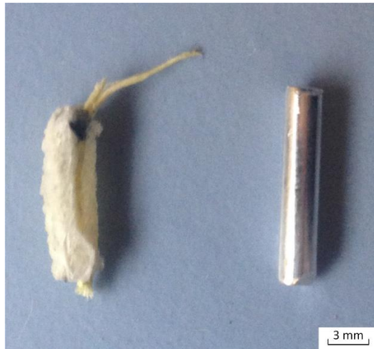
Figure 6-4: A comparison of a tufted resin column (left) and the steel pin used (right).
