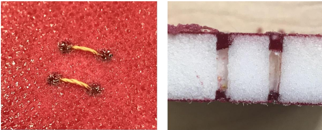
Figure 8-2: Example of lab-scale trials to ‘heal’ needle channel. Left, adhesive film sealing off tuft threads. Right, channel closed-off at top and bottom.
