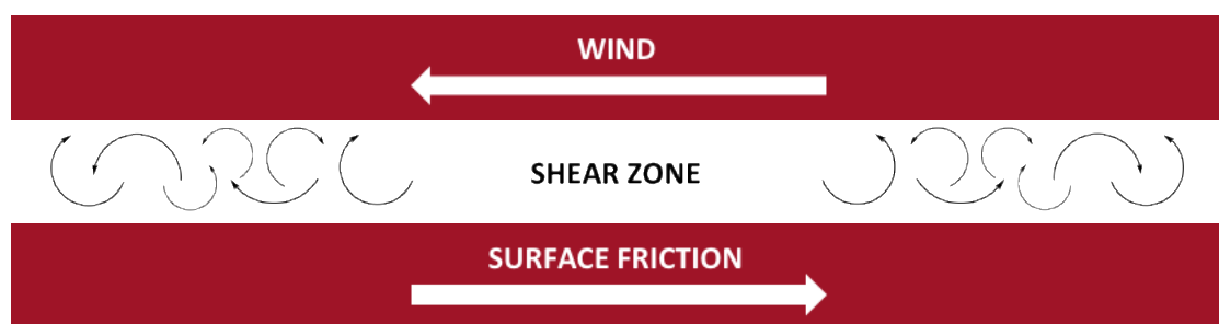
Figure 1.6: Representation of shear stress resulting in turbulence in the ABL.
