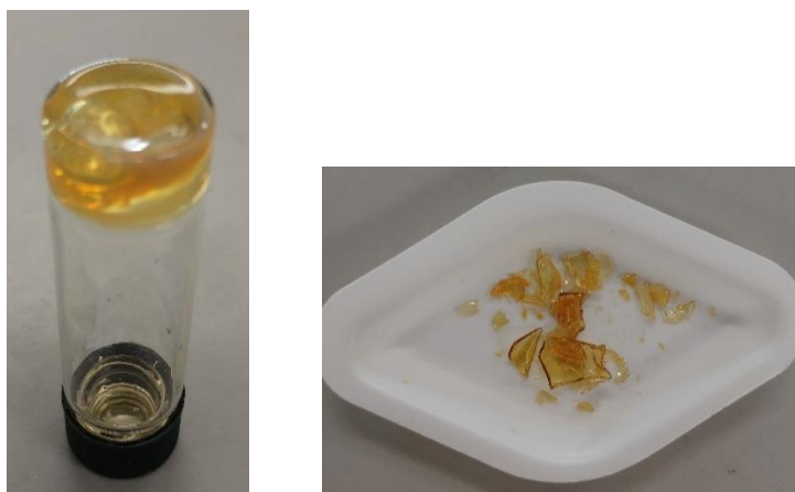
Figure S2.68 Photograph of crosslinked poly(phenylphosphinoborane) after irradiation (left) and after drying under vacuum for 48 h (right).
