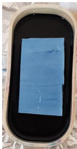
Figure 3-10: Aligned ceramic scaffold infiltrated with blue wax.
