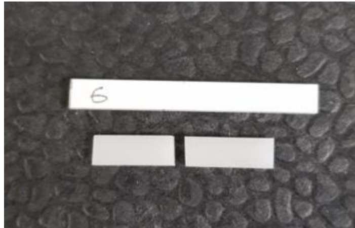
Figure 6-5: Specimens for BCPC4 and Vita Enamic after testing to failure. Note that the BCPC4 specimen is still in one piece, while the Vita Enamic specimen has fractured into two.
