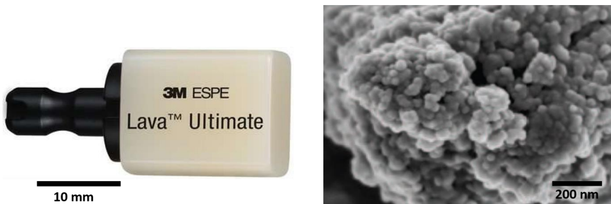
Figure 2-9: Lava Ultimate CAD/CAM block and SEM showing the ceramic nanocluster [134].
