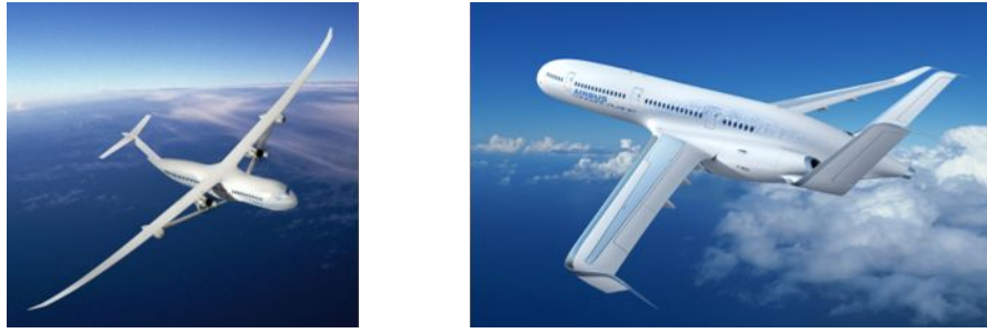
Figure 1.1: Future aircraft concepts that feature high-aspect-ratio wings, from Boeing (left) and Airbus (right).
