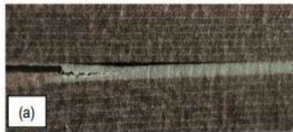
Figure 2.4 - Example of double delamination [9]
