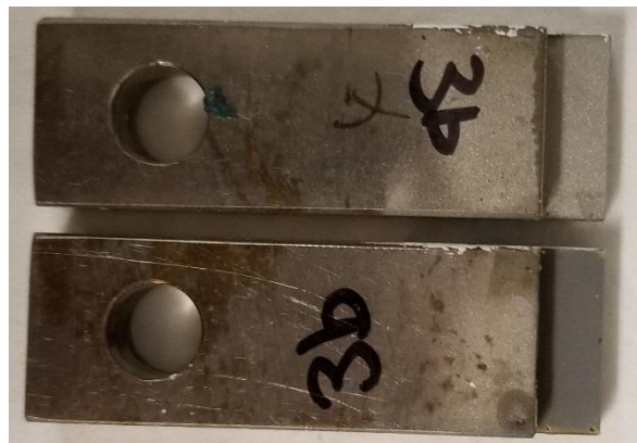
Figure 4.40 - Interfacial failure for shear test at HTW using stainless steel adherends
