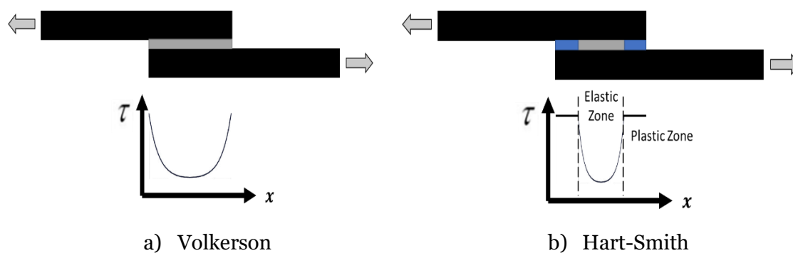
Figure 2.11 – Simplified stress-strain distributions for adhesive joints
