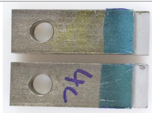
Figure 4.39 - Cohesive failure for shear test at RTD using mild steel adherends
