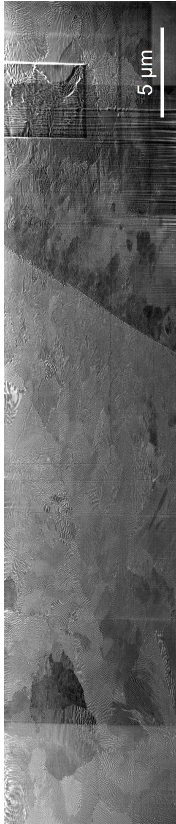
Figure 6.46: FIB-cut cross section of the 500 °C aged UNb7 sample. Within the two original grains in view numerous domains of banded material have formed.
