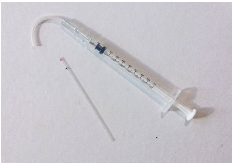
Figure 3 Empty microcapillary tube and equipment used for flushing of blood from the microcapillary tubes. Eppendorf tubes were labelled and pre-filled with 90 \mu l of PBS and opened prior to blood collection; the microcapillary tubes were filled with blood to a 10 \mu l label mark and then placed into the Eppendorf tubes containing the PBS. A 1ml syringe was attached to a 23G butterfly catheter with the tube cut to leave approximately 2.5cm of tubing, as shown. The tubing was attached to the microcapillary tube and PBS flushed through by aspiration and expulsion so that the 100 \mu l of mixed blood and PBS was expelled into the Eppendorf tube, ready for further analysis.
