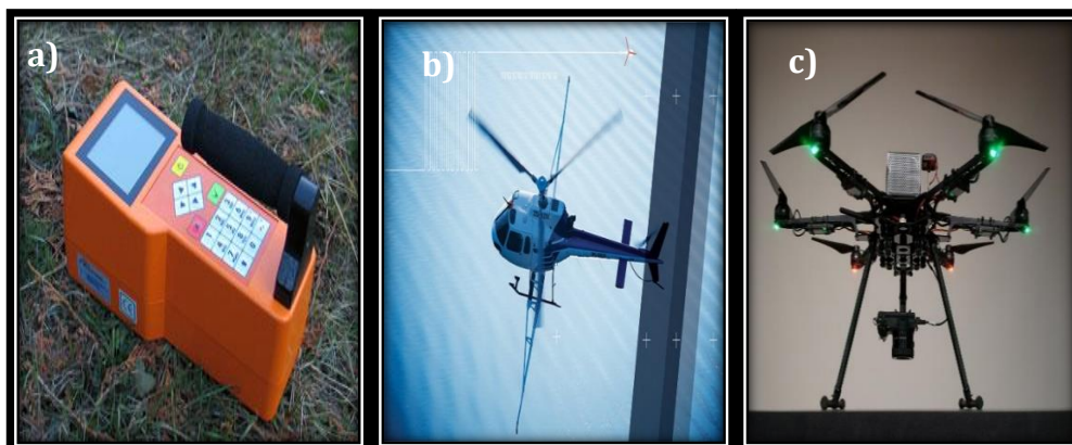
Figure 11. Radioactivity measurements tools a) Handheld (GS) b) TAS c) UAV from [6, 7, 8]
