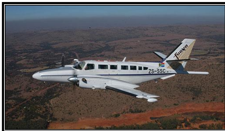
Figure 1. A twin-engine Rheims Cessna F406 aeroplane, fitted with geophysical radiometric survey equipment, used in the Tellus South West survey. Photo courtesy of Fugro Airborne Surveys (Pty) Ltd.
