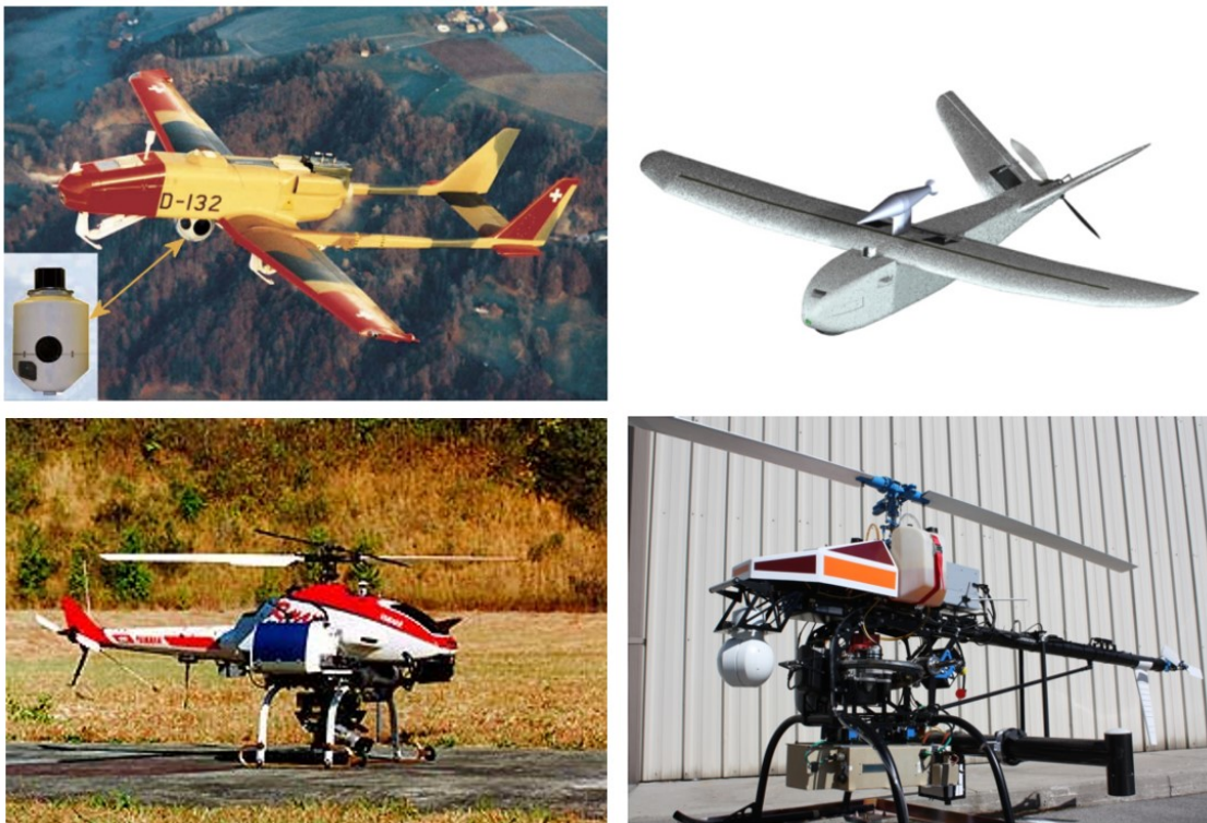
Figure 2.5: Images of various unmanned helicopter and fixed-wing platforms employed for radiation mapping. From (clockwise from top left); Kurvinen et al., (2015), Towler et al., (2012), Pollanen et al., (2009), and Okuyama et al., (2014) [80, 92, 96, 97].
