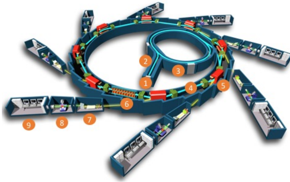
Figure 5.10: Schematic of the component parts of a third generation synchrotron facility such as the Diamond Light Source. Modified from [263].
