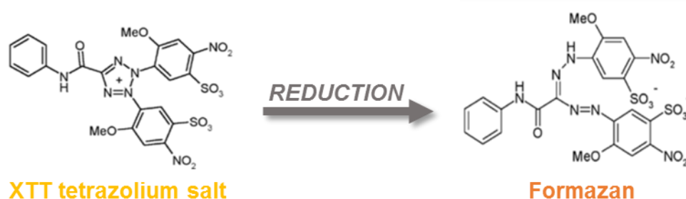
Figure 3.2. Reduction of XTT tetrazolium salt into formazan. Dehydrogenase enzymes in viable cells reduce the slightly yellow XTT tetrazolium salt into the bright orange and soluble dye formazan. Since this reaction relies on the performance of enzymes that are active only in viable cells, formazan absorbance at wavelength 450nm is proportional to the amount of viable cells in the sample.
