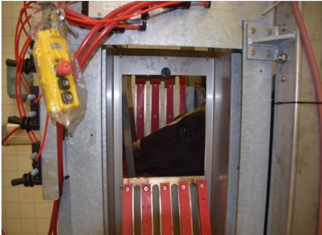
Figure 23. Photograph of the head of a restrained cow showing a side window where EEG and ECG recordings will be taken post stun.
