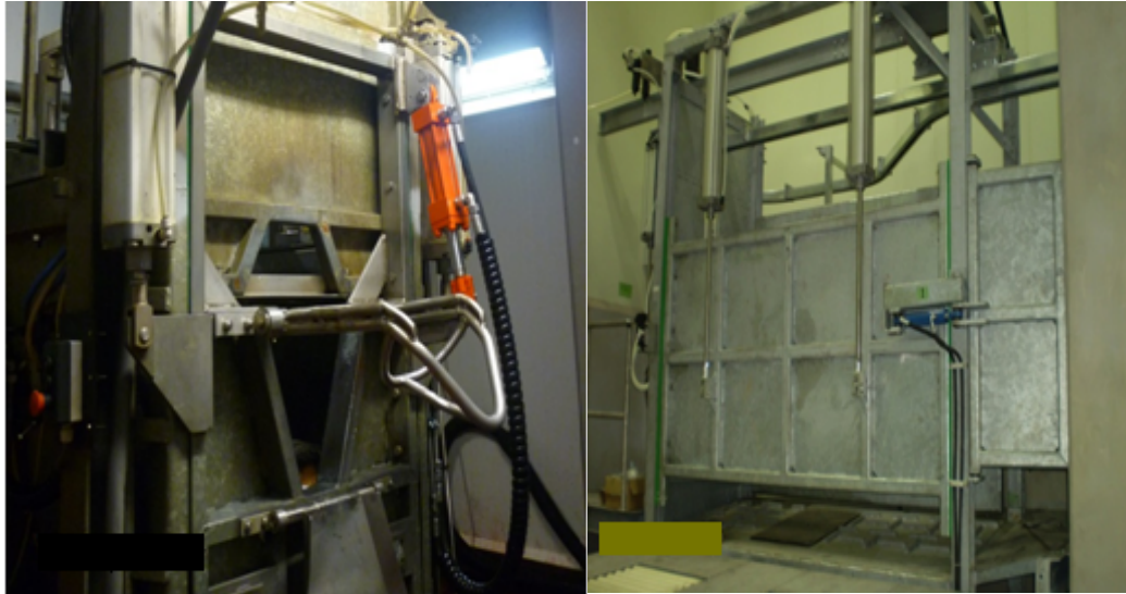
Figure 1. An upright restraint with the chin lift component suitable for use during slaughter without stunning. This may be fitted with a belly lift and back pusher.
