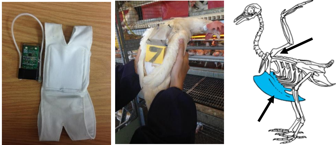
Figure 2.3: Left: Custom made tri-axial accelerometer and vest. Middle: focal bird wearing numbered backpack. Right: Black arrows indicate regions of the hen that the accelerometer sensors were placed
