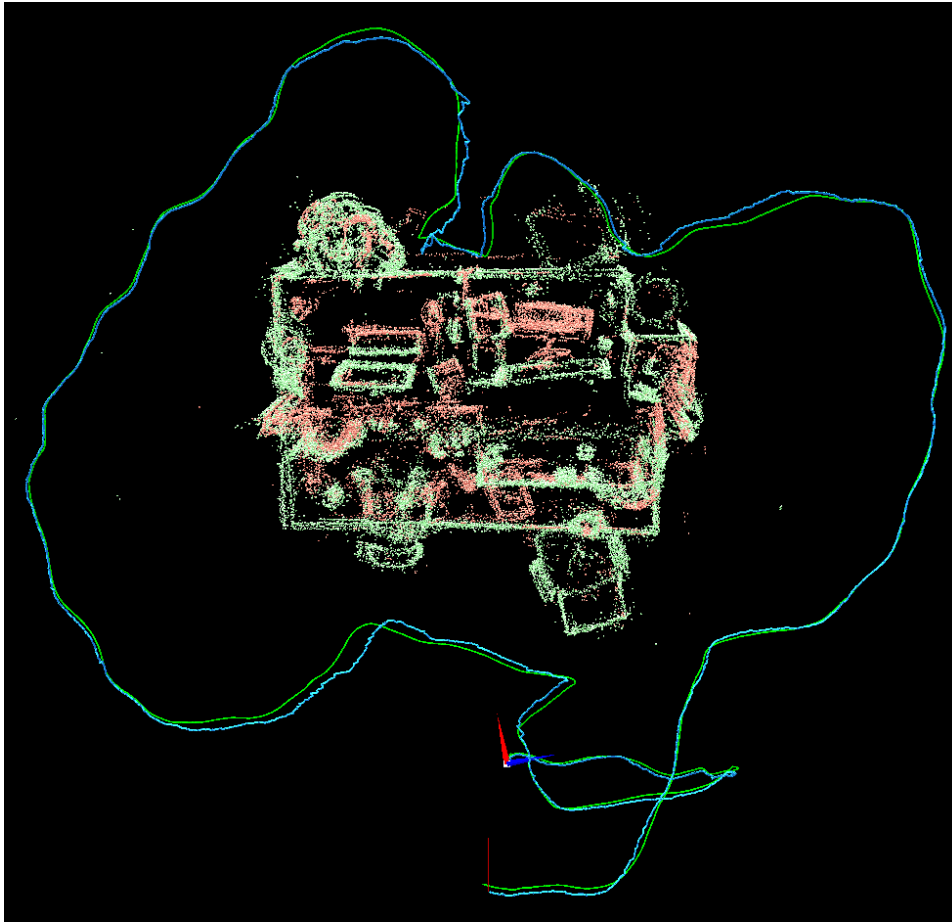
Figure 2.19: Map created by the proposed SLAM from the FR3 "long office household" RGB-D sequence. The ground truth trajectory of the sensor is drawn in green, while that estimated by the SLAM system is shown in blue.
