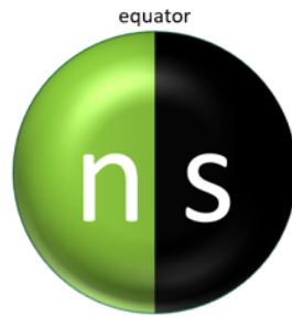
FIGURE 3.15: Presentation of dipole-like formation due to non-uniform charge distribution on the surface
