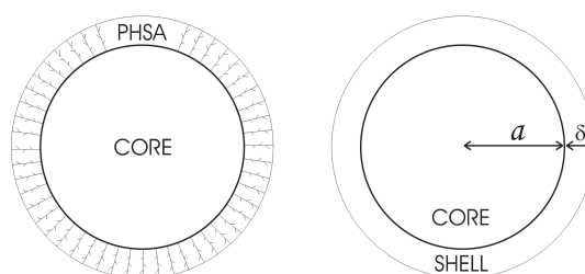
FIGURE 2.1: Illustration of the PMMA colloid with a stabilizing PHSA layer, a = 775 nm and \delta = 10 nm (Finlayson, 2016a)
