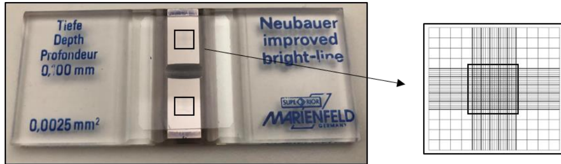
Figure 2-1 Haemocytometer slide for cell counting.
