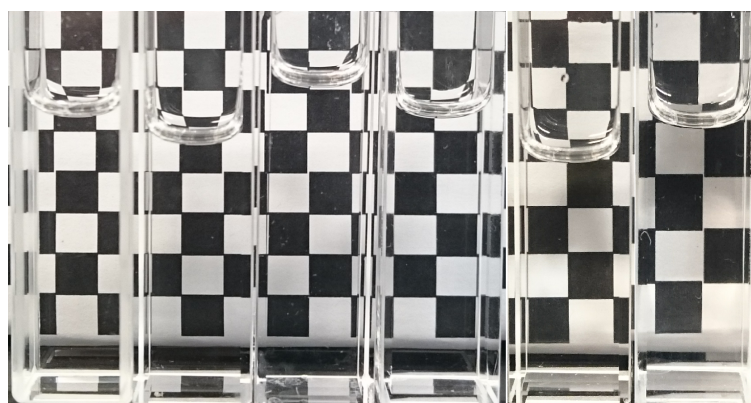
FIGURE 4.14: Vials of TDAT in dodecane at concentrations of (from left to right) 100, 300, 500, 700, 1000 & 1300 \mu\text{M} .
