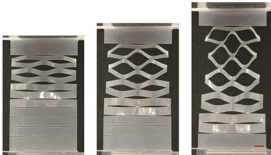
Figure 5.19 The mechanical behavior of the Kirigami structure in Figure 5.18 under three stages of nominal strain: 5 %, 15 % and 30 %. Scale bar: 5 cm.
