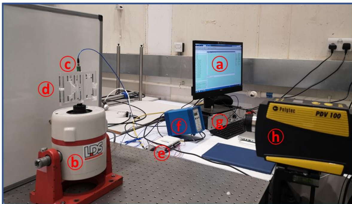
Figure 6.3 Platform setup for the vibration test of the proposed 3D tunable energy harvesting structures. (a) computer for system control and data recording, (b) vibration shaker, (c) accelerometer, (d) the acrylic base with the test structure mounted on it, (e) NI USB-6211 data acquisition device, (f) signal coupler, (g) shaker power amplifier, and (h) laser vibrometer.
