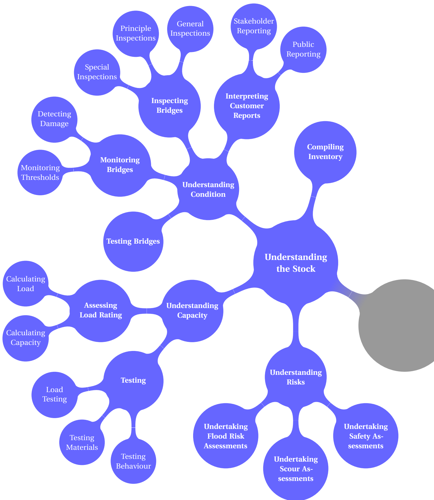
Figure 4.4: Hierarchical Process Model of the Understanding the Stock process within the high-level process of Managing Bridges
