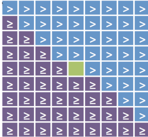
Figure 4.2: The E_T requirement of a trigger tower (green box), relative to its neighbouring trigger towers (purple and blue boxes), in order for a Level-1 jet to be reconstructed about it [6].
