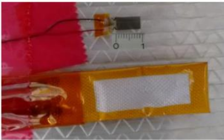
Figure 2.12: Comparison of standard and microscale sensors (smallest scale is mm). Reproduced from [93]
