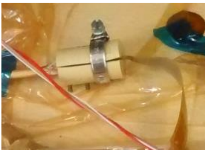
Figure 5.47: Protective cover for connector, with flexible sensor attached. Sensor ~1cm wide.
