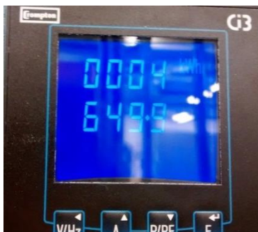
Figure 5.13: The energy monitor on the autoclave electrical cabinet, showing current and total energy usage in kWh. Readings were taken before and after each cure.
