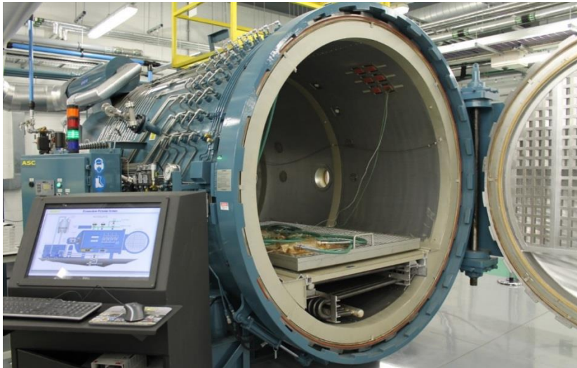
Figure 5.1: The bespoke autoclave (2m internal diameter x 3m length) at the National Composites Centre, with pass-throughs for cure monitoring sensors. The control computer is at the front left. A test part is inside the autoclave, thermocouples attached.
