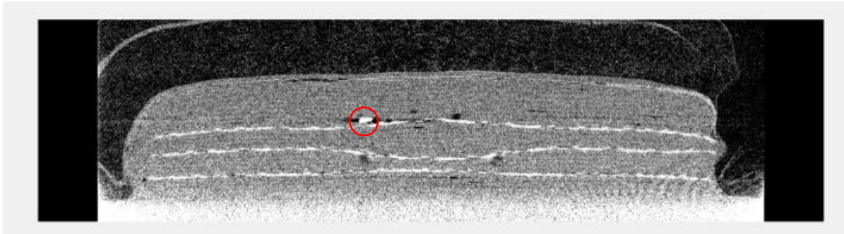
Figure 4.6: Scan 15 (140 minutes), high density contaminant circled
