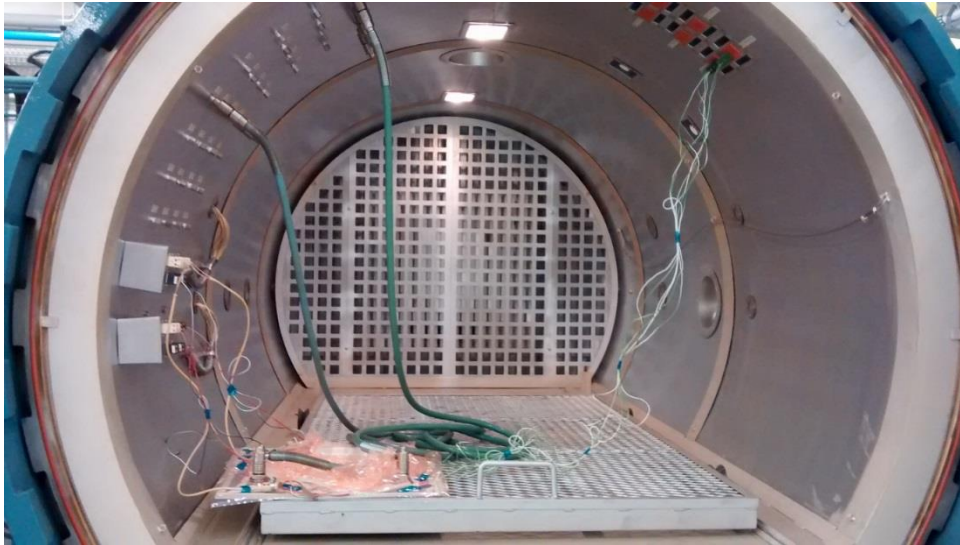
Figure 5.7: A test part connected up to the sensor systems (left), vacuum hoses (left top) and autoclave thermocouples (right), inside the bespoke autoclave. The autoclave has an internal diameter of 3m.
