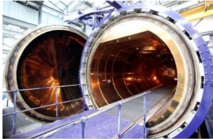
Figure 1.7: Autoclave, 11.2m long x 3.55m diameter [8]. Image from National Composites Centre.[5]
