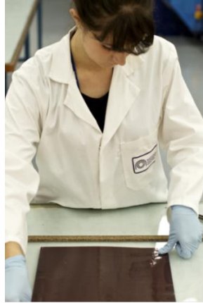
Figure 1.4: Hand layup of prepreg. Image from National Composites Centre.[5]
