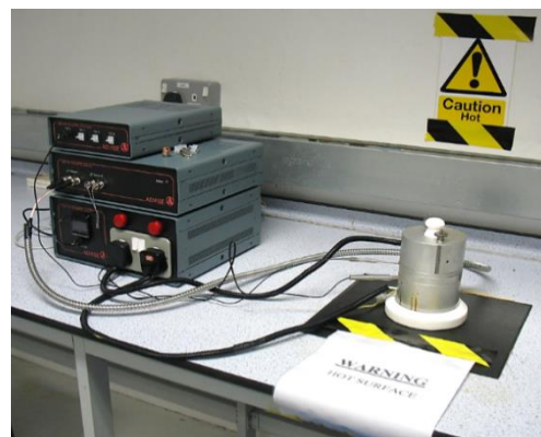
Figure 2.10: A resin cell in use
