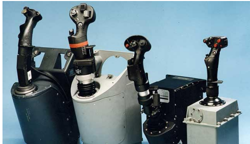
Fig. 1 Aircraft inceptor control systems [3]
