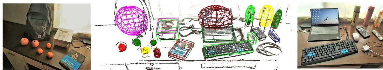
Fig. 12: Results of EAO-SLAM in a real scenario. Left and right: raw images. Middle: semi-dense object-oriented map.
