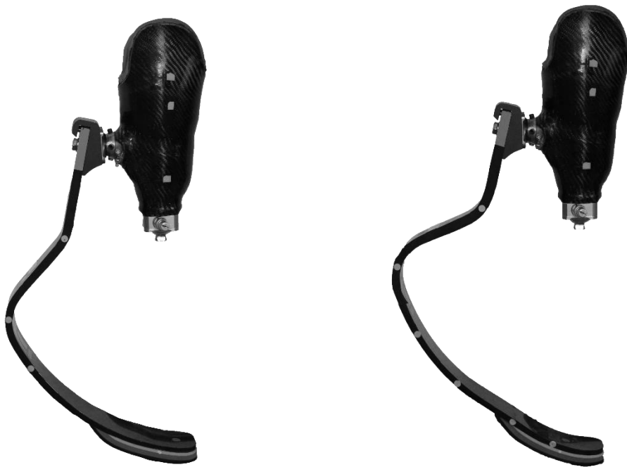
Figure 4 The two prosthetic models used in both for the testing. On the left is the model E prosthetic and on the right the model X prosthetic. (Photo by L. Grobler)
