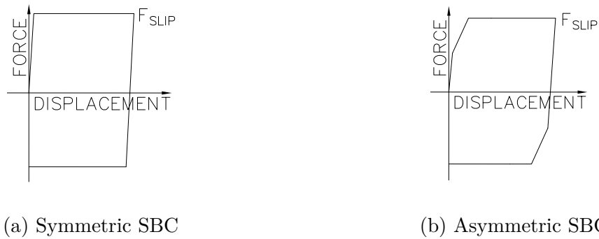
Figure 4.17: Differing hysteretic behaviour for SSBCs and ASBCs (adapted from Loo et al., 2014)
