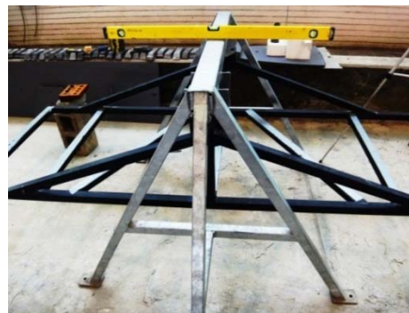
Figure 51: Levelling of the cradle
