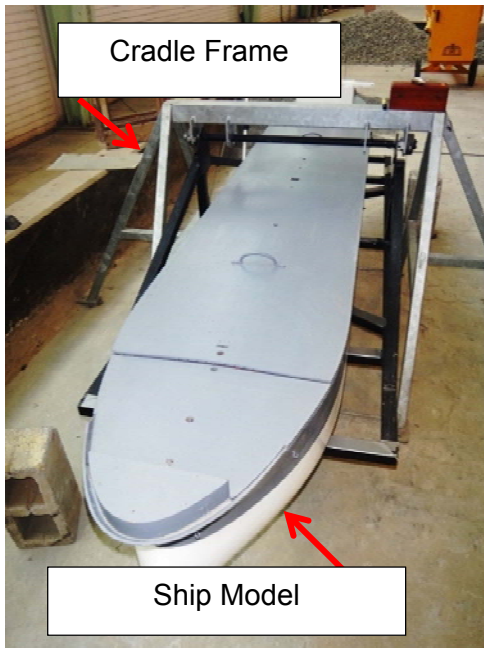
Figure 50: Cradle used for calibration procedures
