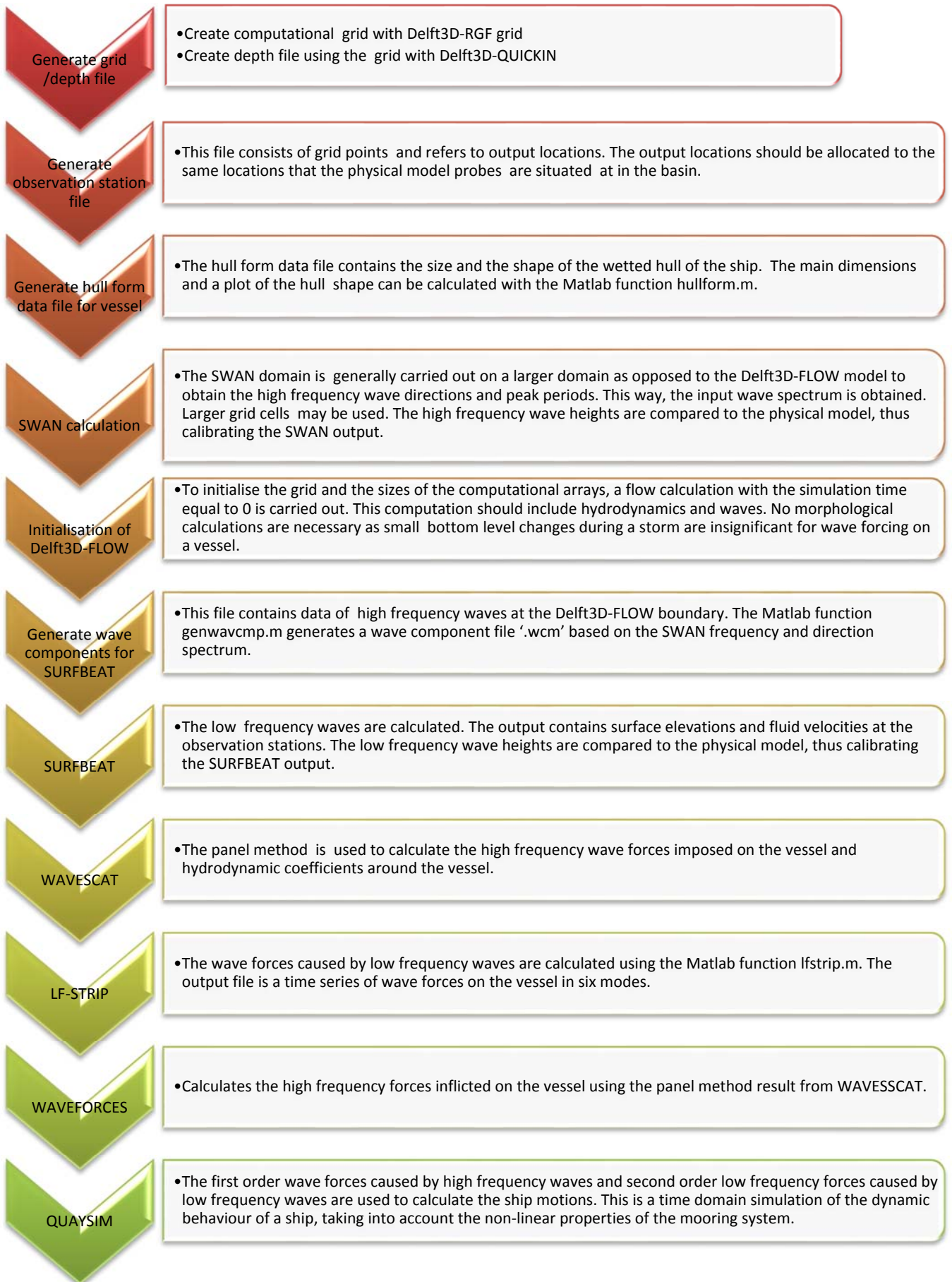
Figure 3b: Detailed description of the computational approach
