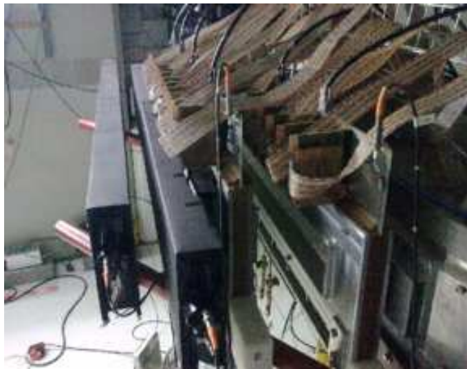
Figure 3.4: The focal plane detector package of the K600 magnetic spectrometer. Two drift chambers and two scintillators are shown.
