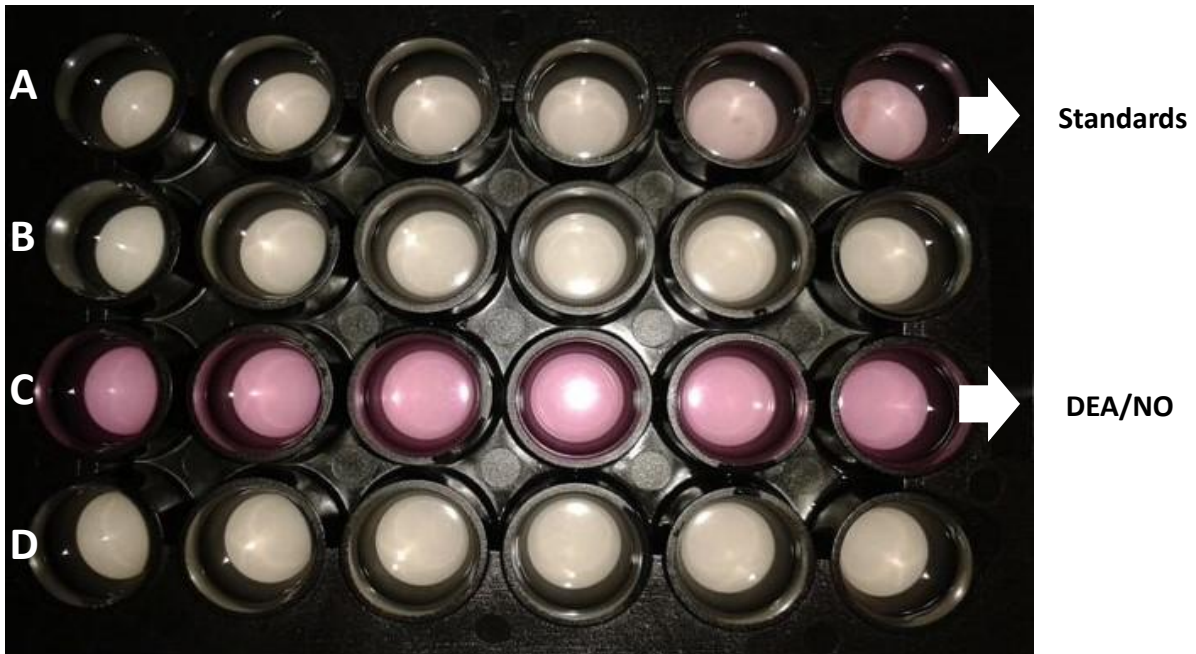
Figure 2.16: A 24 well plate used for Griess reaction experiments. A gradual increase in colour intensity can be observed in row A and represents the increased \text{NaNO}_2 standard concentrations ( 0 \mu\text{M} ; 0.4 \mu\text{M} ; 2 \mu\text{M} ; 4 \mu\text{M} ; 7 \mu\text{M} and 10 \mu\text{M} ). Row C represents the colour reaction observed after treating cells with 10 \mu\text{M} DEA/NO for 3 hours (NO positive control).
