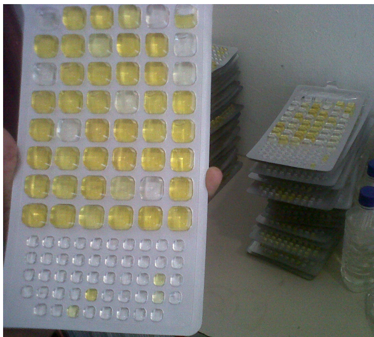
Figure 1: Colilert tray containing a sample that tested positive for the presence of coliforms (yellow colour)
