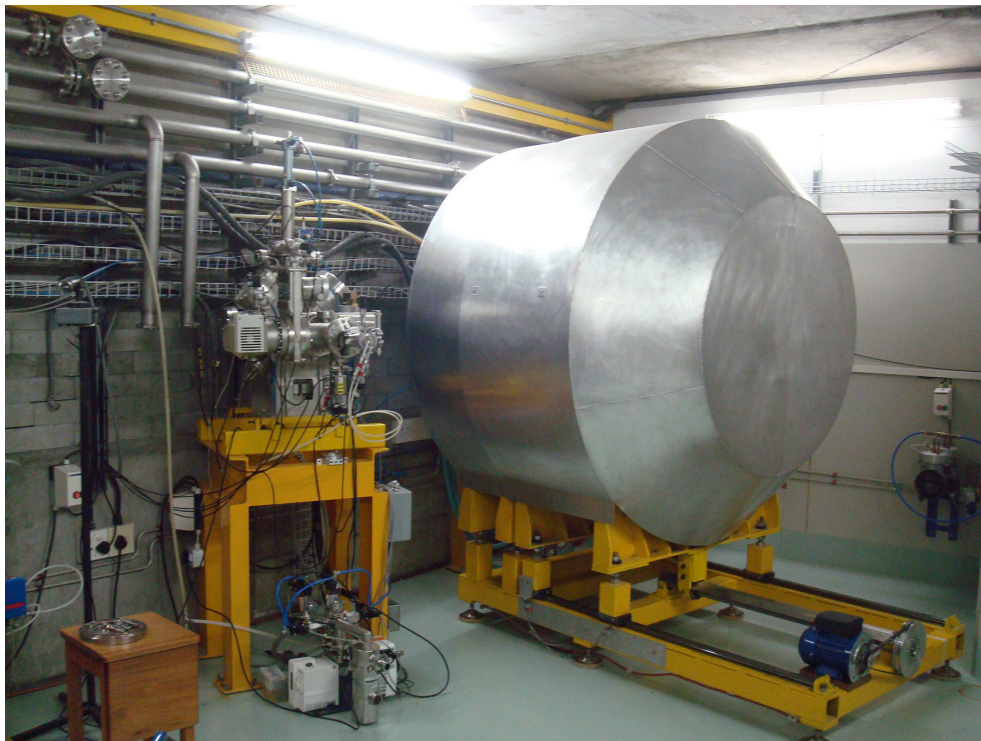
Figure 2.3: Target Station 2 (also called Babe) for irradiating semi-permanent targets.
