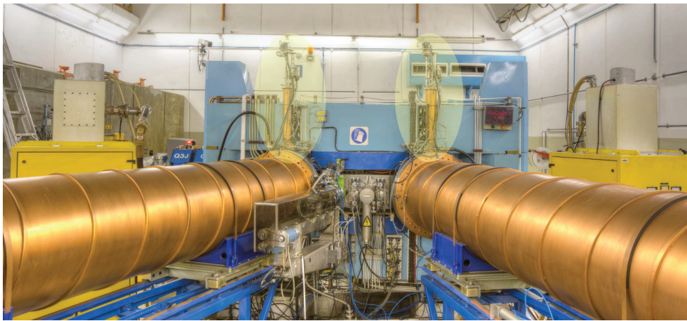
Figure 2.18: Photograph showing the flat-top RF resonators (highlighted) mounted onto the main RF resonators of the light-ion injector cyclotron (SPC1).
