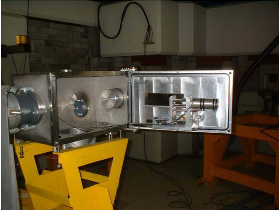
Figure 2.4: The RERAME-II irradiation chamber with the door in an open position. The collimator and vice assemblies are mounted on the door. The guide rods on which the jaws of the vice move ensure positional accuracy. The beamline connects to the chamber on the left of the picture.
