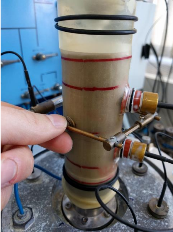
Fig. 1. Unsaturated sample with ICTs and radial strain belt (axial LVDTs yet to be fitted).
