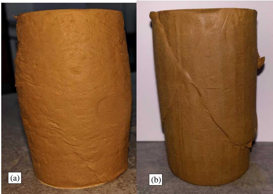
Fig. 4. Photographs of samples after shearing: (a) saturated sample CU350; (b) unsaturated sample CWC-14.5-100.
