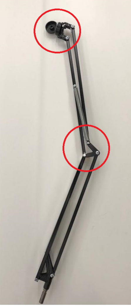
Fig. 4 Manipulator Arm with 2-DoF being manually operated
