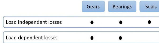
Figure 6: AGB heat loss mechanisms
