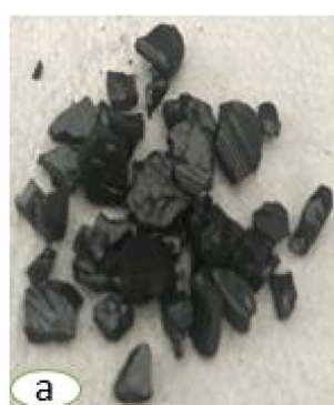
Fig. 2 – Pitch: (a) physical appearance, and (b) chemical components found in pitch-derived from crude oil/petroleum.
