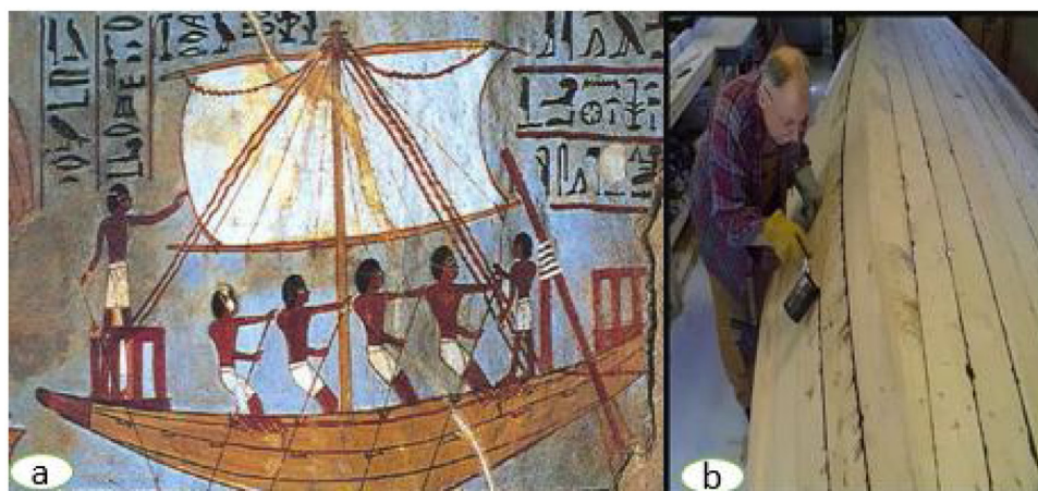
Fig. 1 – (a) Ancient Egyptians used tar/pitch to join wooden plants for shipbuilding, (b) example of pitch being used to waterproof a boat constructed from wooden planks.
