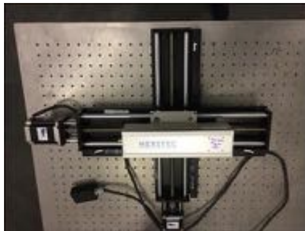
Figure 8.2 HEXITEC detector mounted on the X-Y stage. It is possible to move the HEXITEC up/down and/or left/right by driving the two motors using the Autostep application.
