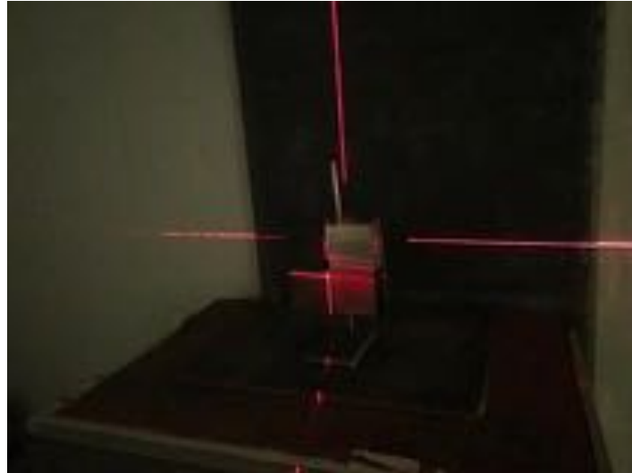
Figure 8.4 Sample alignment to the X-ray source.
