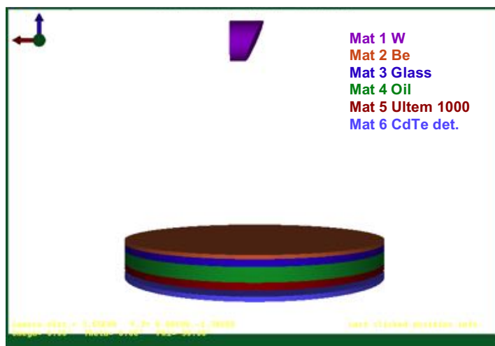
Figure 6.1 The model of the VJT X-ray tube in PENELOPE. The model has been designed with PENGEOM and consists of a tungsten target anode (Mat 1), and four layers of window material in vacuum (beryllium, glass, transformer oil, Ultem 1000, Mat 2-5). A pencil beam of electrons hits the tungsten and then the photons irradiate the layers before being collected by a virtual CdTe detector placed just outside the exit window.
