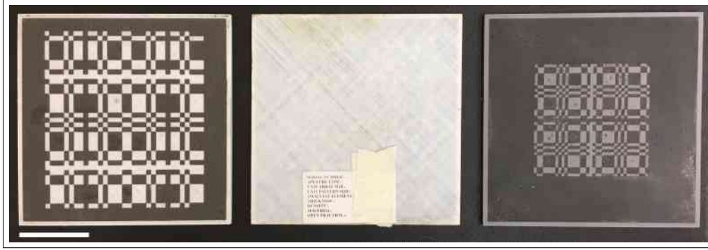
Figure 4.5: 3D Printed TEC CM Examples: (left) a 17 \times 19 TP URA anti-mask, (centre) 3D printed CM view from the back and (right) a cyclic 19 MURA. Note, the feature sizes are extremely different because they are demonstration CMs and the 17 \times 19 TP URA was not used during the project.
