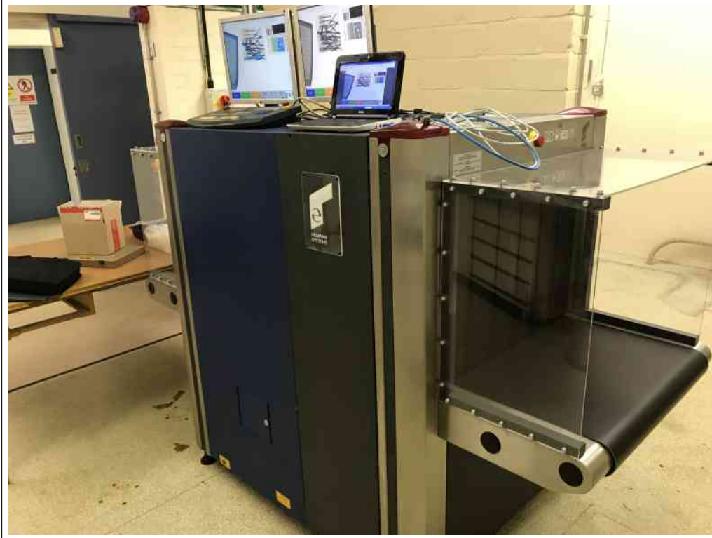
Figure 8.7: Dual Energy X-ray Baggage Scanner: The scanner was used to take all X-ray transmission images.
