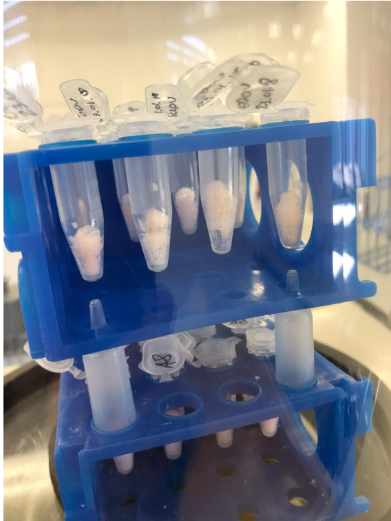
Figure 7. Lyophilized SARS-CoV-2 PV pellets within the sample drying chamber.
