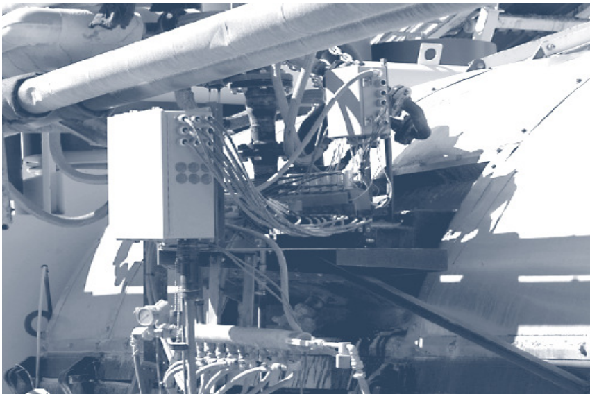
Figure 2.5 Multi-Nozzle Foaming Manifold of Astec (Brock, 2007)
