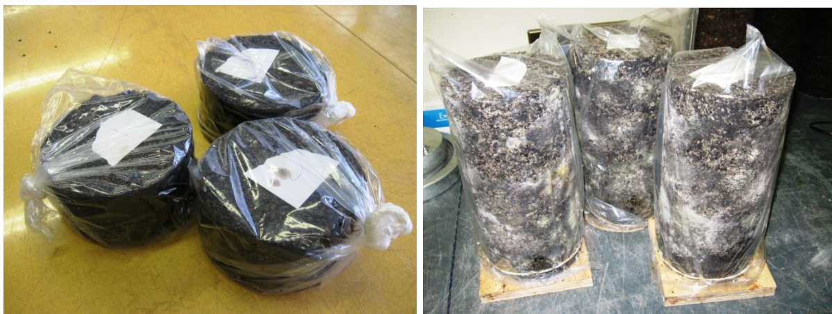
Figure 3.11: ITS and Tri-axial specimens at the end of their curing period.
