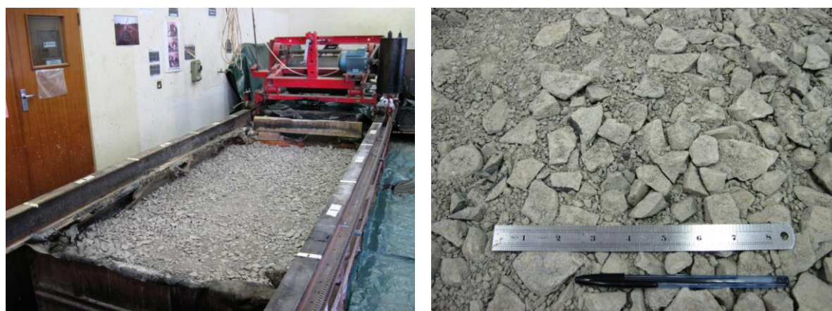
Figure 6.1: Sub-base created in the laboratory with a good crushed stone quality material (Hornfels).
