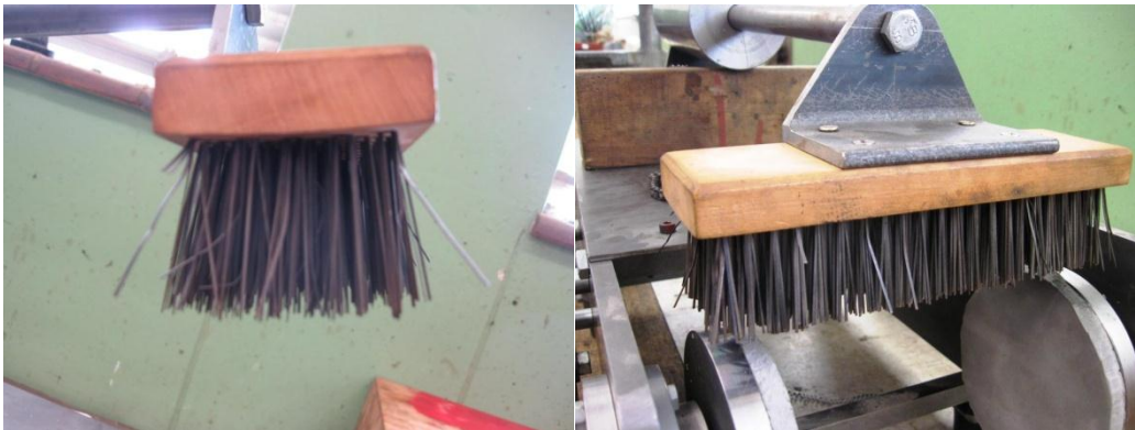
Figure A.1: Wet-Dry Brushing apparatus.
