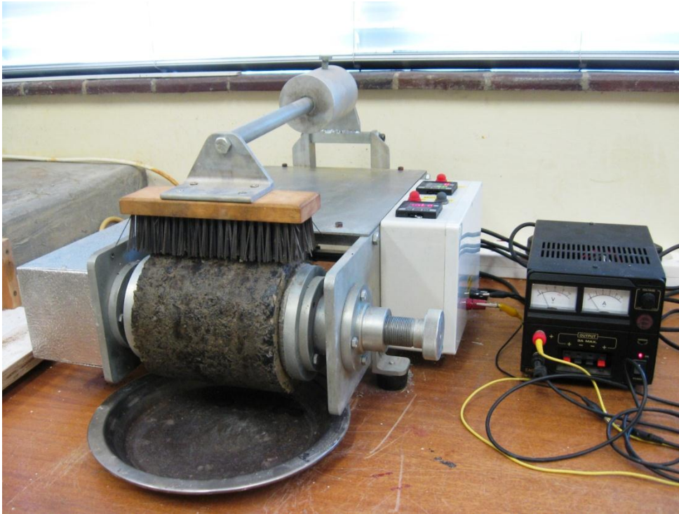
Figure A.1: Wet-Dry Brushing apparatus.
