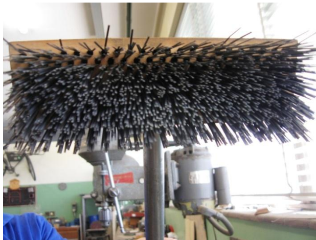
Figure A.2: Details of the wire brush.
