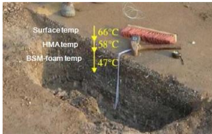
Figure 2.15: Temperature distribution of distressed pavement structure including BSM-foam as a base layer (Jenkins and Twagira, 2008).
