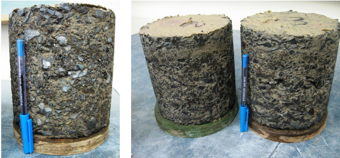
Figure 5.19: Effect of erosion of wet-dry brushing on BSMs mixtures.
