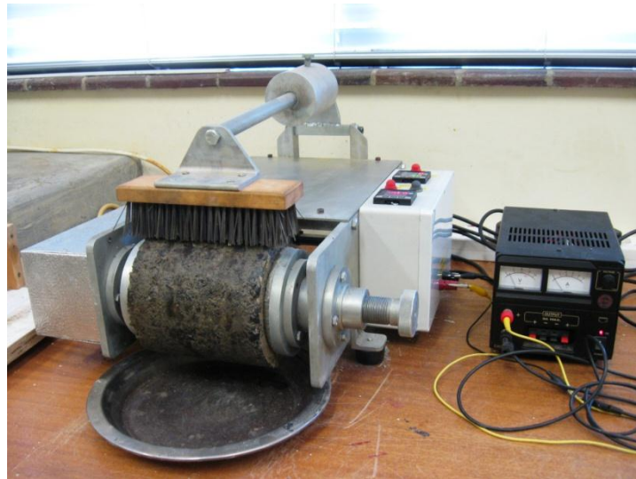
Figure 5.5: Mechanical brushing apparatus at Stellenbosch University.
