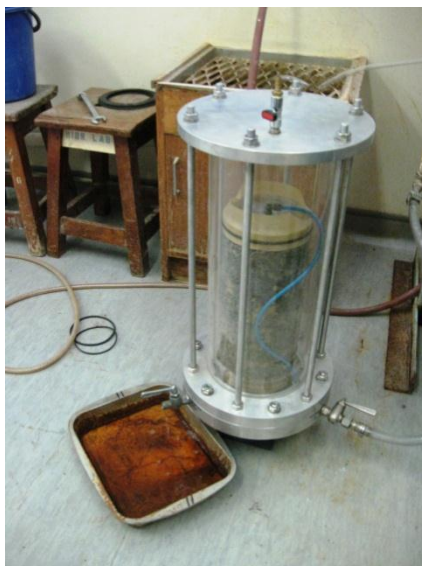
Figure 5.2: Permeability test in the laboratory at Stellenbosch University.
