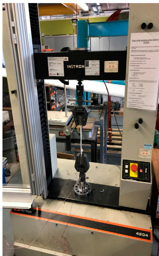
Figure 6. Instron testing machine carrying out testing.
