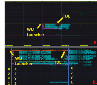
Fig. 14. Implementation layouts of the DSWU TDC. a) Overview. b) Clock regions (X2Y1 ~ X2Y3).
