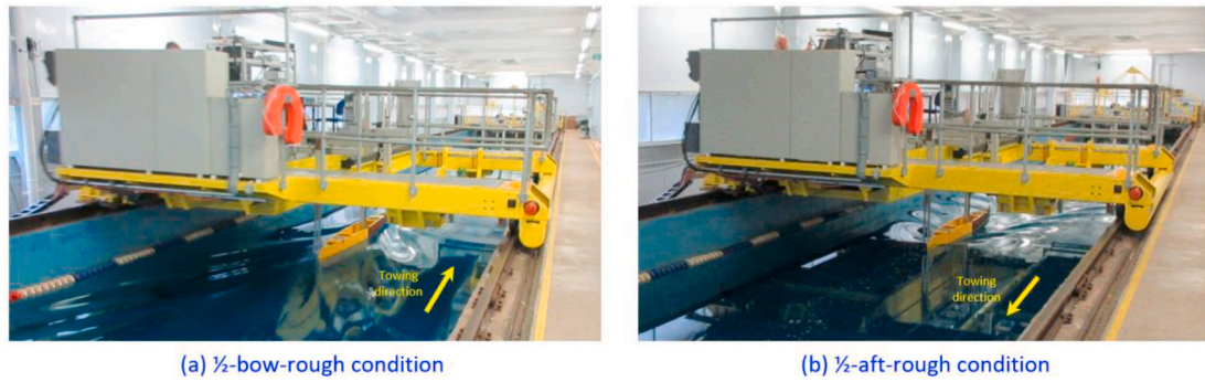
Fig. 3. The towing carriage of the Kelvin Hydrodynamics Laboratory and the Wigley model; (a) 1/2-bow-rough condition, (b) 1/2-aft-rough condition.
