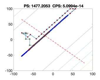
Fig. 2 Functioning and performance of standard Pattern Search (PS) and its enhanced version that exploits the mathematical knowledge about eigenvectors (CPS)
