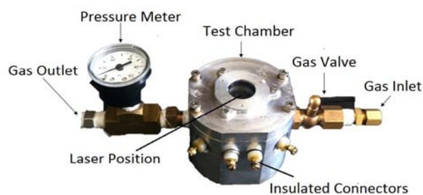
Figure 2: Chamber used for testing the sensor. Gas inlet and outlet pipes are on the side with the laser fixed on the top.
