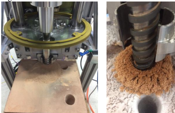
Figure 1: UPCD sampling dry (L) and saturated (R) Locharbriggs sandstone
