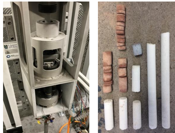
Figure 2: P-RAID architecture (L) and core samples of sandstone, limestone and microgabbro (R)
