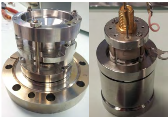
Figure 3: (left) The impact tolerant penetrator deployable mass spectrometer (right) the mole deployable mass spectrometer
